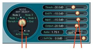
You can also add or remove nodes by using the Node Edit Selector knob and toggling the Active Node switch. Click on the knob and move the mouse either vertical or horizontal to rotate it and select a node. Use the Active Node switch to turn a node on or off.
